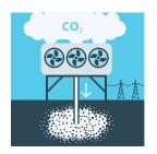
**Principle:** with DACCS, CO<sub>2</sub> is mechanically filtered out of the atmosphere and stored beneath the ground. Here, carbon is captured with the aid of a technical system instead of by plants.
